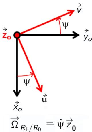
$$\vec{\Omega}_{R_1/R_0} = \dot{\psi} \vec{z}_0$$
