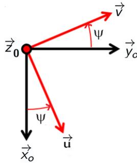
$$\vec{v} = \cos \psi \vec{y}_0 - \sin \psi \vec{z}_0 \quad \vec{u} = \cos \psi \vec{x}_0 + \sin \psi \vec{y}_0$$
