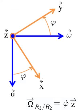
$$\vec{\Omega}_{R_3/R_2} = \dot{\varphi} \vec{z}$$
