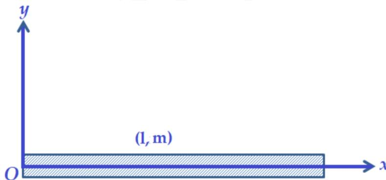
$$I_{/Oy} = \int_{(S)} x^2 dm = \int_{(S)} x^2 \rho dx = \rho \int_0^l x^2 dx = \rho \left[ \frac{x^3}{3} \right]_0^l$$
