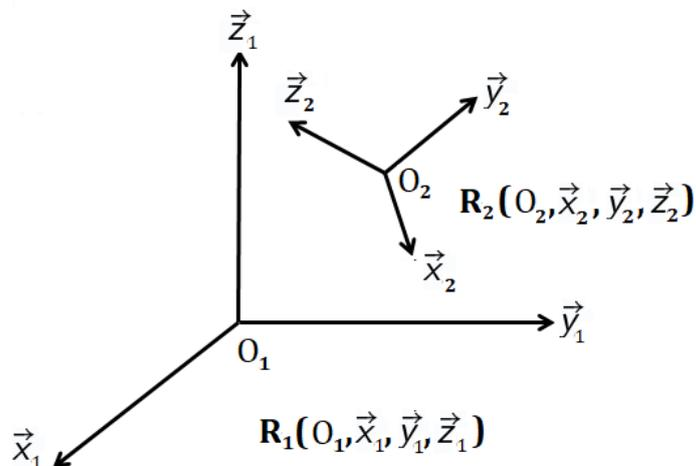
$$\vec{V}(M) = \frac{d\overrightarrow{O_1M}}{dt} /_{R_1} = \frac{d\overrightarrow{O_1O_2}}{dt} /_{R_1} + \frac{d\overrightarrow{O_2M}}{dt} /_{R_1}$$
