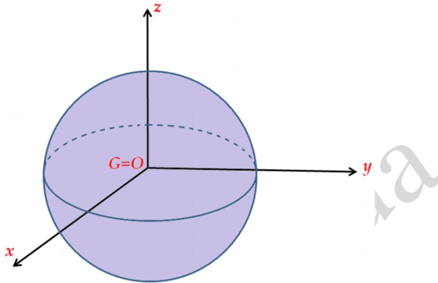
$$I_{/O} = \int_{(S)} (x^2 + y^2 + z^2) dm, \quad I_{/Ox} = I_{/Oy} = I_{/Oz} = \int_{(S)} (x^2 + y^2) dm$$
