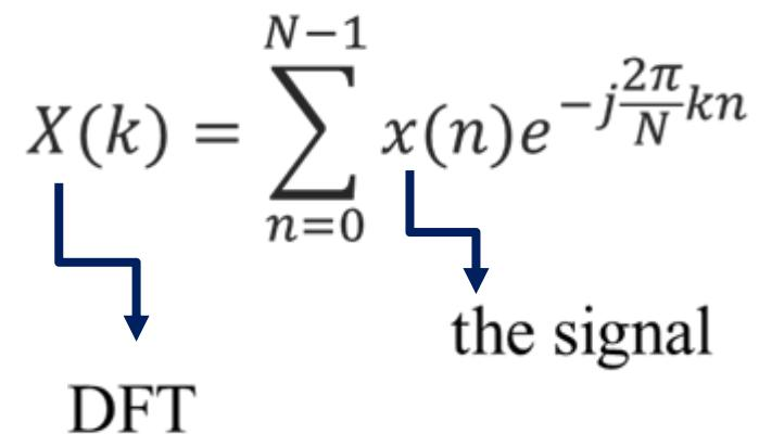
**Example:** Applying the DFT to an image allows for frequency analysis, helping to identify periodic patterns or noise.
