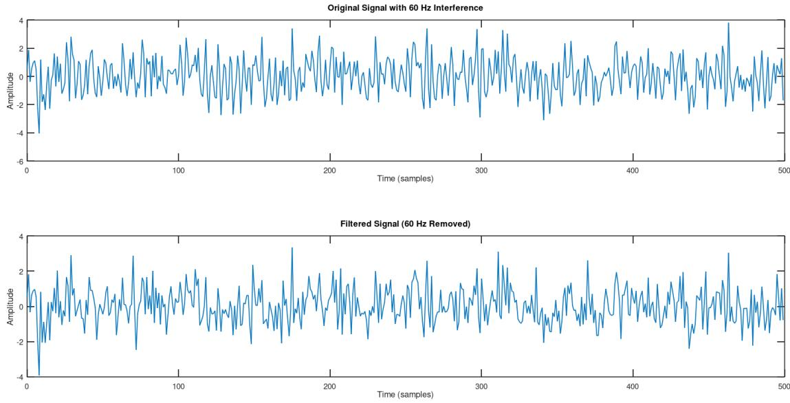
To remove the 60 Hz interference, we will design a **Notch Filter** (a type of band-stop filter) with a narrow bandwidth around 60 Hz. The goal of this filter is to attenuate frequencies around 60 Hz without significantly affecting the rest of the signal spectrum.
