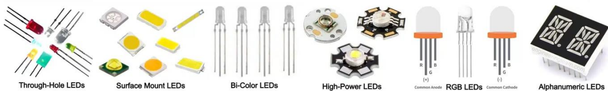
Fig 7: Different type shapes of LED
