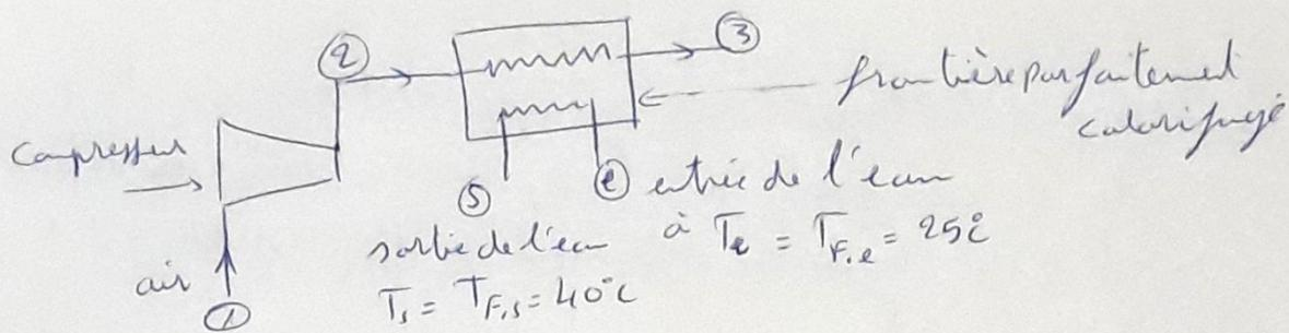
$$\dot{Q}_{eau} = \dot{Q}_{es} = \dot{m}_{eau} c_e (T_{F,5} - T_{F,e})$$
