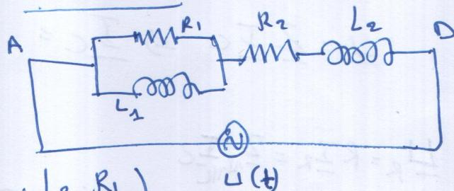
b)  $\underline{Z}_{AD} = 2R_2 \left(1 + j \frac{L_2 \omega_0}{R_2}\right) = 2R_2 \left(1 + j \frac{L_2 R_1}{R_2 L_1}\right)$
