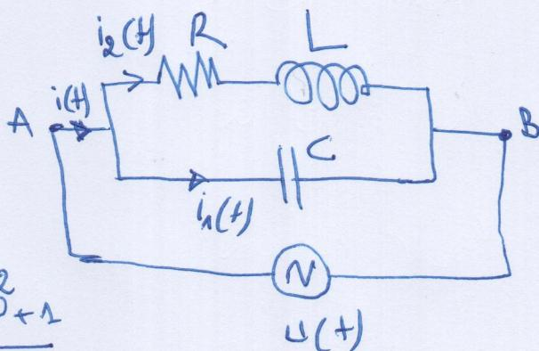
2.  $U = Z_{AB} I \Rightarrow I = \frac{U}{|Z_{AB}|} = U \sqrt{\frac{(1 - \omega^2 LC)^2 + (\omega RC)^2}{R^2 + \omega^2 L^2}}$
